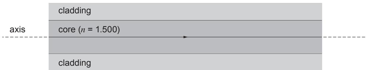
(i) Show clearly that a light pulse travelling along the axis of the fibre takes  $8.0\mu\text{s}$  to travel through 1.6 km of fibre. [2]
