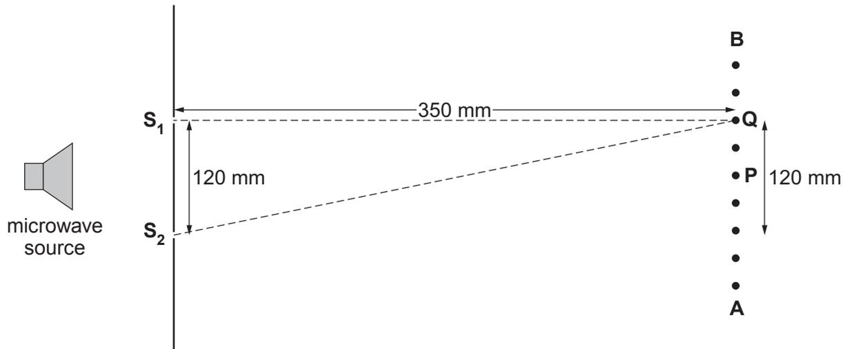
A microwave sensor which is moved along the line **AB** detects maxima at the points shown as dots. One of these points, **Q**, is directly in front of  $S_1$ .
